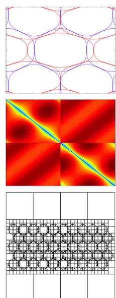
**Figure 2:** (Top) Deformation of a patch of grains in a pure shear flow. (Middle) Dense Stokeslet matrix generated by the BIE. (Bottom) Adaptive domain partitioning of smaller grain-melt aggregate for FMM expansions.
